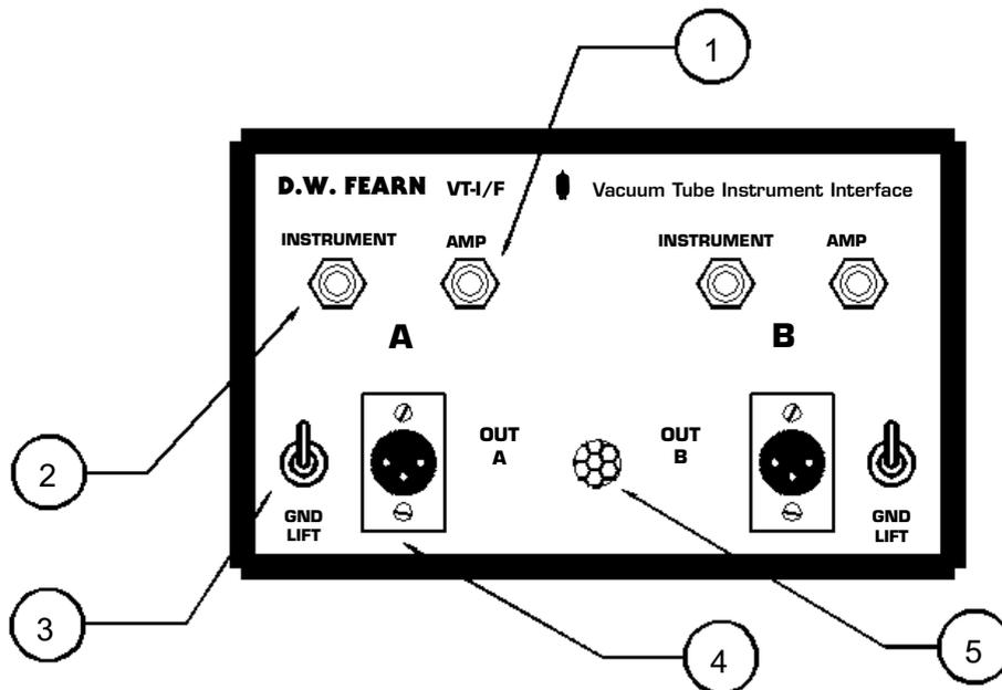
**Figure 2. VT-I/F Front Panel Controls and Connections**
