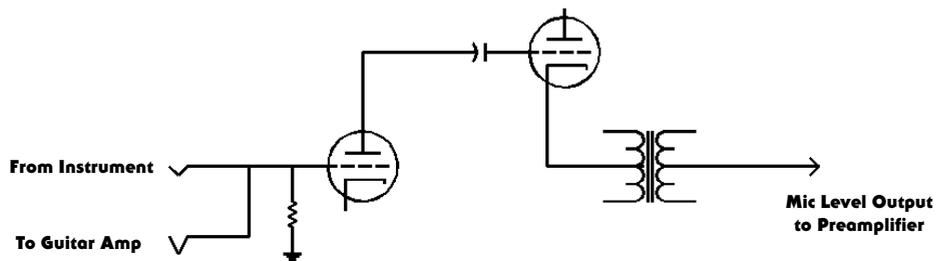
**Figure 3. VT-I/F Block Diagram**
