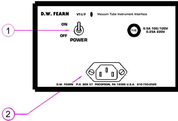
**Figure 1. VT-I/F Rear Panel Connections and Controls**
