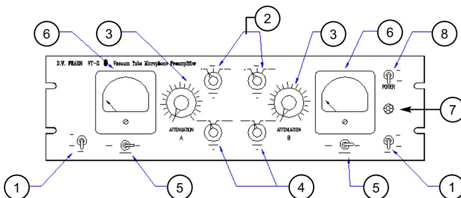
**Figure 2. VT-2 front panel controls and indicators**
