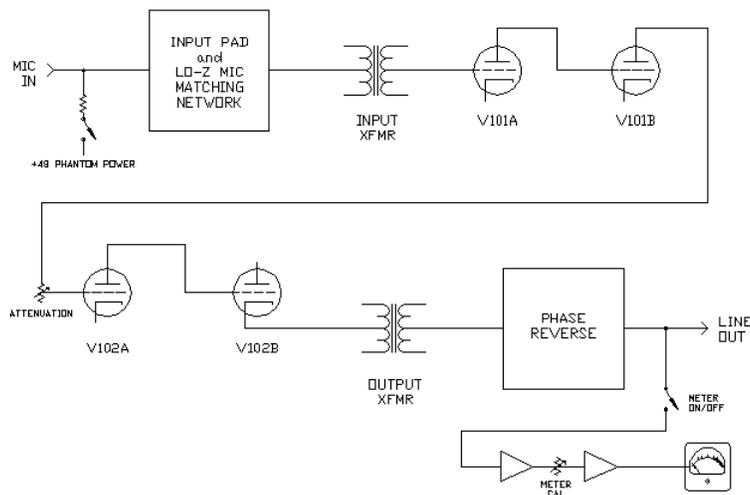
**Figure 4. VT-1/VT-2 Block Diagram (one channel shown)**
